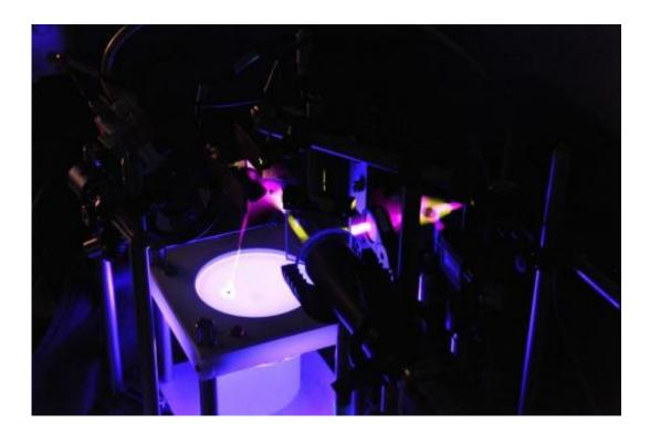
This composite image shows a laser being aimed at a walking fly using the FlyMAD system. Credit: Matt Staley and Dan Bath, JFRC, HHMI
