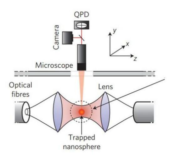
Experimental schematic. Silica spheres are levitated in a dual-beam optical tweezer inside a vacuum chamber. Light of wavelength 1,064 nm is coupled into lenses from single-mode optical fibres, creating an optical trap. The motion of the levitated sphere is monitored with a camera and a QPD. Credit: (c) *Nature*, DOI: 10.1038/nnano.2014.82
