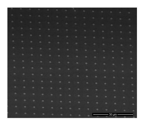
This is a scanning electron microscope image of nickel islands on silicon protected by a titanium dioxide film. Credit: Shu Hu/Caltech
