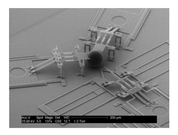
This SEM (scanning electron microscope) image shows the nanoinjector next to a latex bead the same size as an egg cell. You can see the size of the nanoinjector and its lance compared to a cell. Credit: Brian Jensen/BYU
