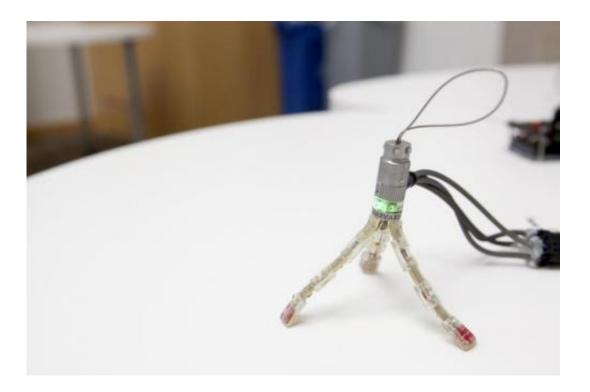
Crafted in a 3D printer and outfitted with rubberized pressure sensors, this inexpensive device designed at Harvard offers surgeons a confident grip on delicate tissue. Credit: Eliza Grinnell, Harvard SEAS.
