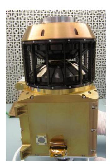
The MAVEN Solar Wind Ion Analyzer will study ions in the Martian atmosphere, a key component for better understanding the planet's evolution. Credit: University of Colorado at Boulder LASP
