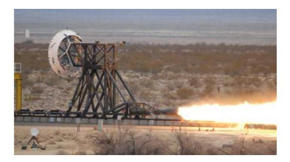
NASA conducted a series of rocket sled tests in 2012 to see how well the lander design slowed down a test vehicle. Credit: JPL
