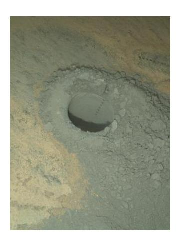
The Mars Hand Lens Imager on NASA's Curiosity Mars rover provided this nighttime view of a hole produced by the rover's drill and, inside the hole, a line of scars produced by the rover's rock-zapping laser. The camera used its own white-light LEDs to illuminate the scene on May 13, 2014. Credit: NASA/JPL-Caltech/MSSS
