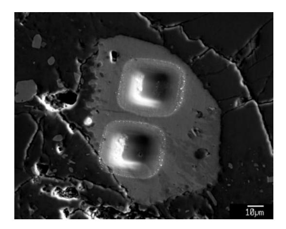
Secondary electron image of pits left by ion microprobe analyses of a heterogeneous apatite grain in Apollo sample 14321, 1047. Water has now been detected in apatite in many different lunar rock types. Credit: K.L. Robinson, HIGP.
