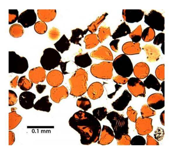
Optical micrograph of pyroclastic glass beads in Apollo sample 74220, 383, the famous "orange soil". Water was first detected by Saal et al., 2008 in glass beads similar to these. Credit: G.J. Taylor, HIGP
