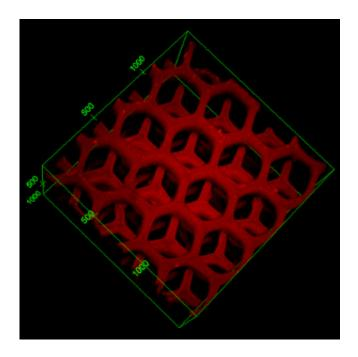
Nanoengineers have developed a 3D printed device inspired by the liver to remove dangerous toxins from the blood. The device, which is designed to be used outside the body like dialysis, uses nanoparticles to trap pore-forming toxins that can damage cellular membranes and are a key factor in illnesses that result from animal bites and stings, and bacterial infections. Credit: University of California - San Diego
