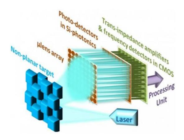
This is a conceptual vision for an integrated 3D camera with multiple pixels using the FMCW laser source. Credit: Behnam Behroozpour
