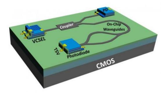
This is a 3-D schematic showing MEMS-electronic-photonic heterogeneous integration. Credit: Niels Quack
