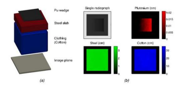
Simulated inspection of a layered, baggage-like object that contains a thin, shielded plutonium wedge (a) (not to scale). A single energy radiograph is shown in (b), along with the material estimations from the adaptive inverse algorithm that indicate an equivalent of color vision (by material) for a single-view radiograph using spectral X-ray detector data.
