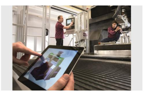
For a deeper look into outer space, astronomers need a new generation of optical telescopes. To produce the ultra-precise large-scale mirrors needed for these instruments, OptoTech designed an 86-metric-ton special-purpose machine.
