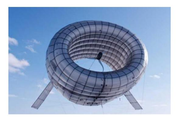
The Buoyant Air Turbine (or BAT), developed by Altaeros Energies, uses an inflatable shell to float 1,000 to 2,000 feet above ground, where winds blow five to eight times stronger, and more consistently, than winds at tower level. Credit: Altaeros Energies
