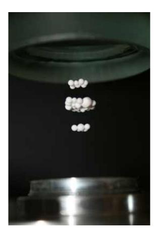
Sound engineering: complex sonotweezers can manipulate and arrange many small particles simultaneously. Credit: Professor Bruce Drinkwater, Bristol University
