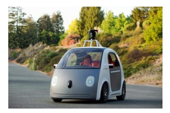
Google plans to build and launch onto city streets a small fleet of subcompact cars that could operate without a person at the wheel. Actually, the cars wouldn't even have a wheel. Or gas and brake pedals. The company says the vehicles will use sensors and computing power, with no human needed.
