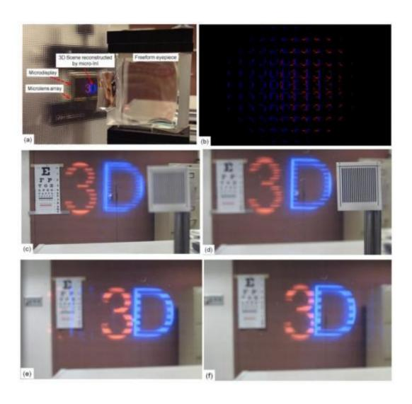
(a) This is the set-up of the experiment. (b) To create a 3-D scene, the micro integral imaging display combines many views of the scene from different perspectives. Here, a 3-D depiction of the characters "3D" is decomposed into its
