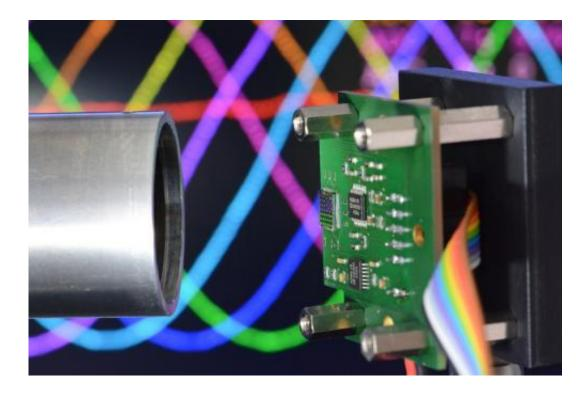
The polarization sensor that measures the angle of rotation mounted on the test board. On the left: A shaft with integrated polarizing film. Credit: Fraunhofer IIS
