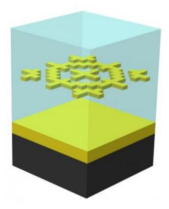
Overall layers of the metamaterial absorber are shown. The black layer is the substrate, solid green layer is palladium, transparent blue layer is polyimide, broken green layer is the patterned layer and the transparent blue layer is again polyimide to seal and protect. Credit: Bossard, Penn State
