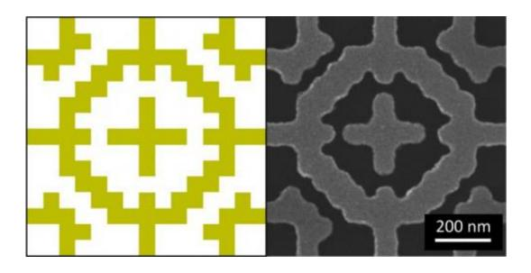
(1) This is a drawing of the metamaterial absorber pattern. (r) This is an actual metamaterial absorber pattern. Credit: Bossard, Penn State
