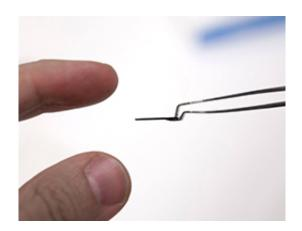
A small, light and effective micro fuel cell generates electrical energy from hydrogen, ethanol and methanol. Gianmario Scotti has developed economical and rapid methods for the purpose of fabricating micro fuel cells in his doctoral research.
