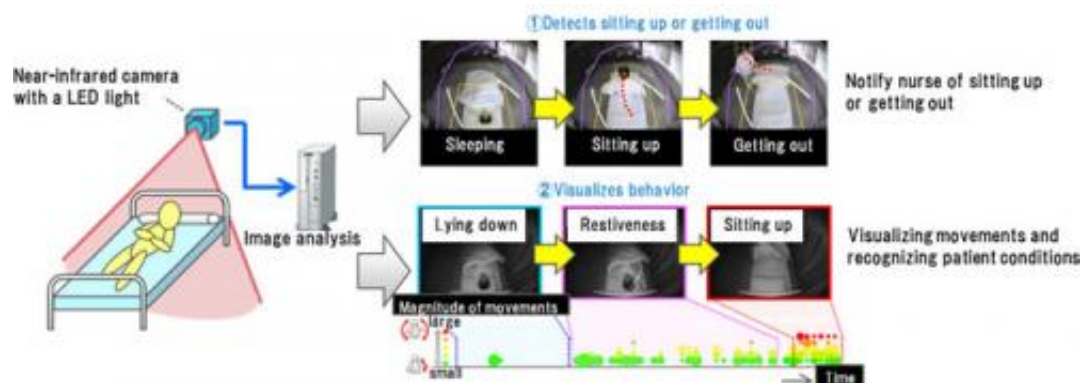
Figure 1: Technology of recognizing patient status using a camera
