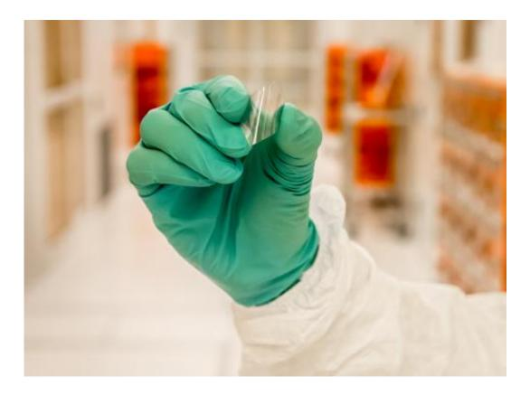
The thin-film transistor is flexible, transparent and performs just as well as commercial versions. Displayed is an array of transistors – each of which are just 10 atomic layers thick. Credit: Mark Lopez/Argonne National Laboratory.
