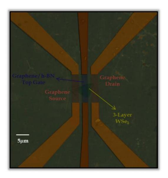
A scanning electron microscope image of the thin-film transistor, fabricated using single-atom-thick layers of graphene and tungsten diselenide, among other materials. The white scale bar shows 5 microns, which is about the diameter of a strand of spider silk. Credit: Saptarshi Das.
