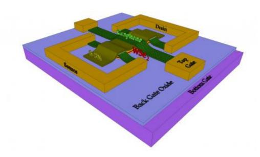
This illustration shows the landscape of the thin-film transistor created by Argonne scientists, which is just 10 atomic layers thick. The transistor is transparent and can be bent without loss of performance. Credit: Saptarshi Das.
