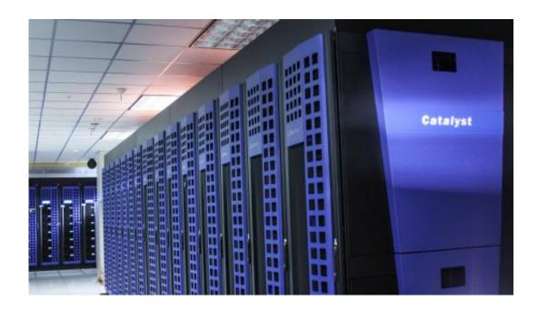
The Catalyst supercomputer at Lawrence Livermore employs a Cray CS300 architecture modified specifically for data-intensive computing. The system is now available for collaborative research with industry and academia.
