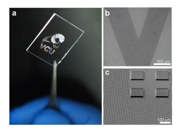
A wide range of patterns and features can be formed from silk proteins at small length scales. For example, microscale dots can be printed on glass to form a silk hologram. Credit: Vamsi Yadavalli, Ph.D./VCU.
