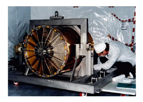
Curved mirrors stacked within one of three optical modules of ESA's XMM-Newton telescope. Each one contains 58 mirrors with a total telescope optical surface of more than 120 m<sup>2</sup> – bigger than a tennis court. Credit: ESA
