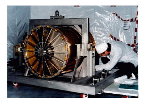
Curved mirrors stacked within one of three optical modules of ESA's XMM-Newton telescope. Each one contains 58 mirrors with a total telescope optical surface of more than 120 m2 – bigger than a tennis court. Credit: ESA
