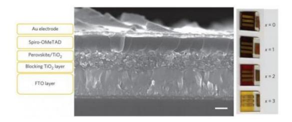
Representative cross-sectional SEM view of a completed photovoltaic device with CH3NH3SnI3 perovskite. Credit: (c) *Nature Photonics*, DOI: 10.1038/nphoton.2014.82
