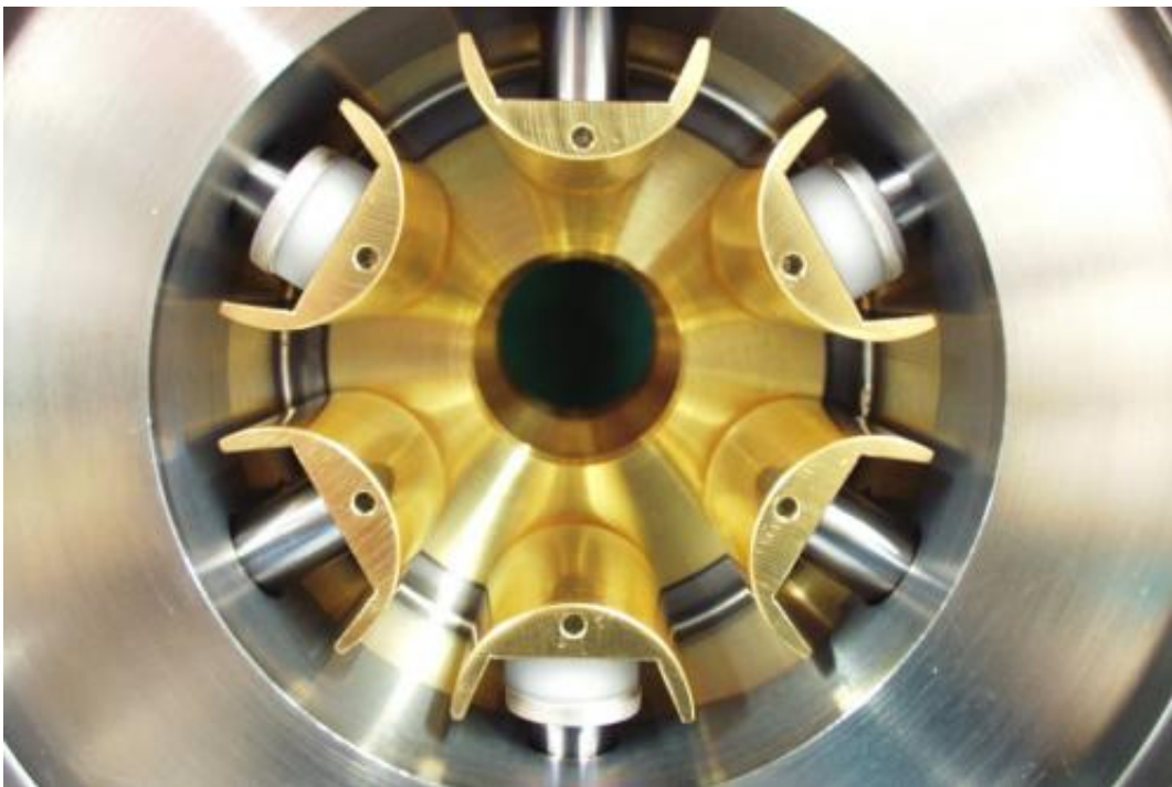
Part of the DFMS (double focusing mass spectrometer): the individual components were joined together by means of vacuum brazing and electron
