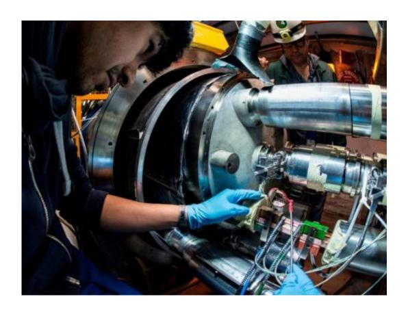
An engineer uses a small mirror to inspect a shunt on an interconnection between superconducting magnets on the Large Hadron Collider Credit: Maximilien Brice/CERN
