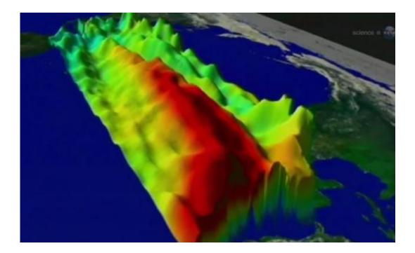
Every ten days, the NASA/French Space Agency Jason-2 satellite maps all the world's oceans, monitoring changes in sea surface height, a measure of heat in the upper layers of the water. Because our planet is more than 70% ocean, this information is crucial to global forecasts of weather and climate.
