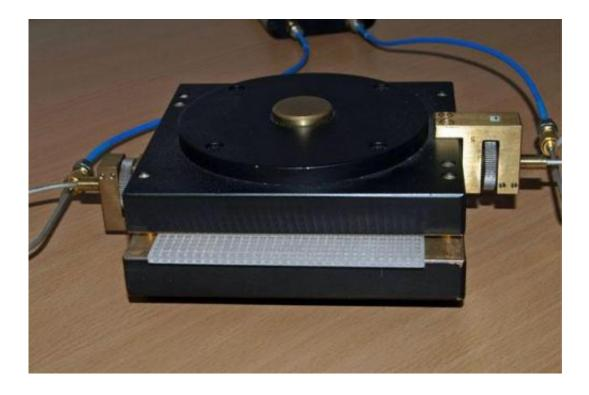
A sample of heterogeneous substrate being measured for effective permittivity in the lab at Loughborough.
