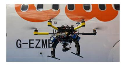
A demonstration of an aircraft inspection by a drone. Credit: easyJet
