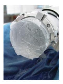
Ice core in the drill head. Past variations of local surface temperatures in polar regions are reconstructed by analysing ice cores drilled in Greenland and Antarctica. Credit: Laurent Augustin
