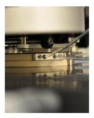
This is a photograph of the high temperature liquid cell attached to the atomic force microscope (MFP-3D-SA, Asylum Research, Santa Barbara, CA). The cell is equipped with inlet/outlet ports for liquid injection and a heating element that regulates temperatures as high as 300 C. Credit: University of Houston
