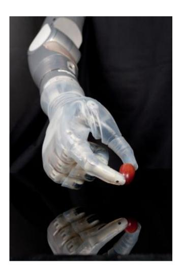
The DEKA Arm System is capable of handling objects as delicate as grapes and eggs and also manipulating power tools, such as a hand drill.
