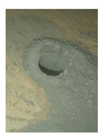
The Mars Hand Lens Imager on NASA's Curiosity Mars rover provided this nighttime view of a hole produced by the rover's drill and, inside the hole, a line of scars produced by the rover's rock-zapping laser. The hole is 0.63 inch (1.6 centimeters) in diameter. The camera used its own white-light LEDs to illuminate the scene on May 13, 2014. Credit: NASA/JPL-Caltech/MSSS
