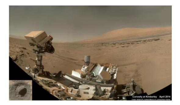
Curiosity snaps selfie at Kimberley waypoint with towering Mount Sharp backdrop on April 27, 2014 (Sol 613). Inset shows MAHLI camera image of rovers mini-drill test operation on April 29, 2014 (Sol 615) into "Windjama" rock target at Mount Remarkable butte. Mastcam color photo mosaic assembled from raw images snapped on Sol 613, April 27, 2014. Credit: NASA/JPL/MSSS/Marco Di Lorenzo/Ken Kremer – kenkremer.com
