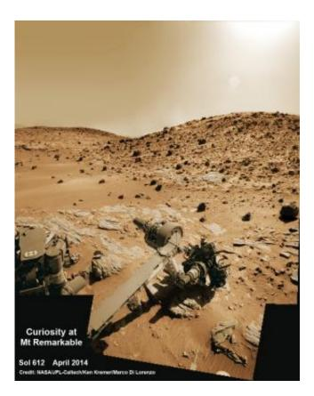
Multisol composite photo mosaic shows deployment of Curiosity's rovers robotic arm and APXS X-ray spectrometer onto the 'Winjana' rock target at Mount Remarkable for evaluation as missions third drill target inside Gale Crater on Mars. The colorized navcam raw images were stitched together from several Martian days up to Sol 612, April 26, 2014. Credit: NASA/JPL-Caltech/Ken Kremer – kenkremer.com/Marco Di Lorenzo
