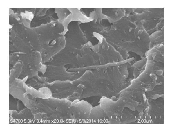
A Scanning Electron Microscopy (SEM) image of the new ultra-strong polymer reinforced with carbon nanotubes. Credit: IBM
