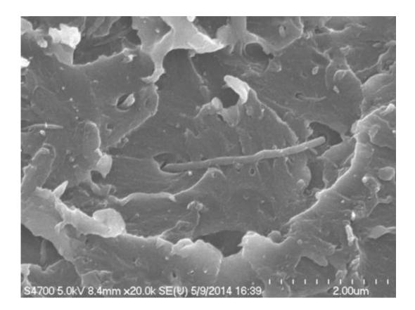
A Scanning Electron Microscopy (SEM) image of the new ultra-strong polymer reinforced with carbon nanotubes. Credit: IBM
