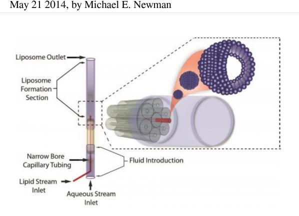
Schematic of the NIST/University of Maryland 3D-microfluidic hydrodynamic focusing device for manufacturing vesicles known as liposomes. Phospholipids dissolved in alcohol flowing through the center capillary (red) mix with a waterbased buffer solution added through the six surrounding tubes. Liposomes are created downstream from the convergence point. Credit: NIST
