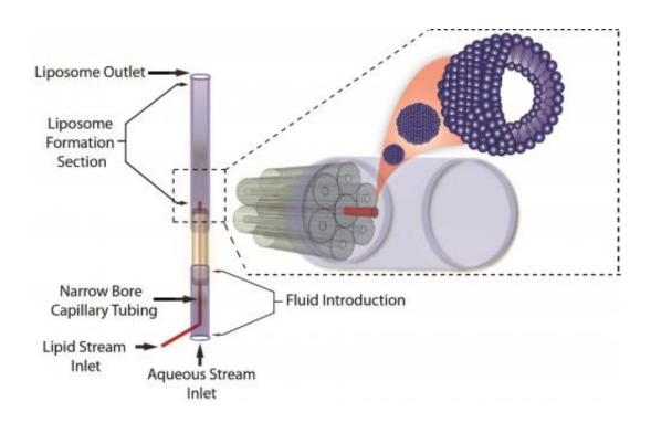
Schematic of the NIST/University of Maryland 3D-microfluidic hydrodynamic focusing device for manufacturing vesicles known as liposomes. Phospholipids dissolved in alcohol flowing through the center capillary (red) mix with a water-based buffer solution added through the six surrounding tubes. Liposomes are created downstream from the convergence point. Credit: NIST
