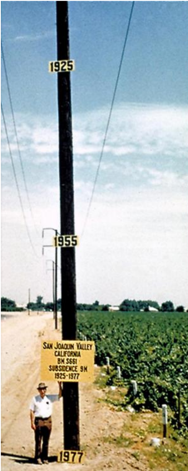
This photo shows the approximate location of maximum subsidence in the United States, identified by research efforts of Dr. Joseph F. Poland (pictured).
