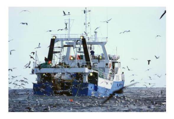
A hake trawler with thousands of birds in attendance is shown. The orange buoy and bird scaring lines are visible off the stern of the vessel. Credit: Ross Wanless
