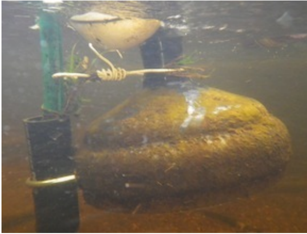
A bubble trap collecting freshwater bubbles from Allequash Creek. Credit: Center for Limnology/John Crawford
