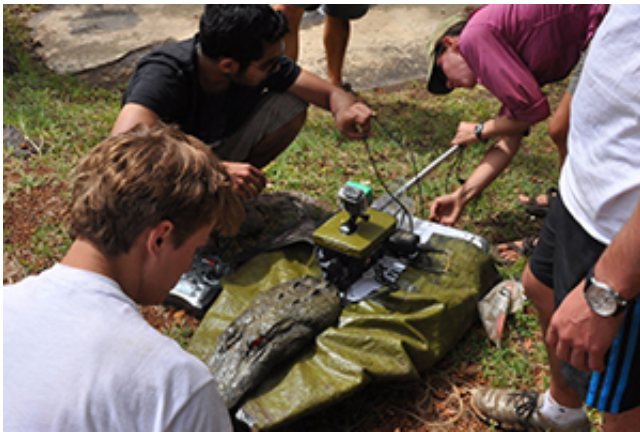
Autonomous airboats, disguised to look like crocodiles
