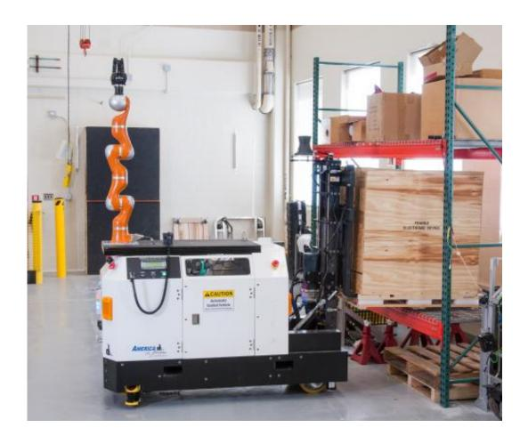
Operating autonomously, the NIST AGV is removes a crate from an industrial rack. AGV is used in the development of safety and performance metrics and test methods for the manufacturing applications. Credit: Bostelman/NIST
