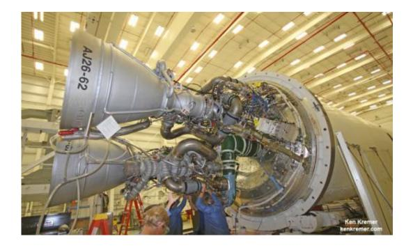
Orbital Sciences technicians at work on two AJ26 first stage engines at the base of an Antares rocket during exclusive visit by Ken Kremer/Universe Today at NASA Wallaps. These engines powered the successful Antares liftoff on Jan. 9, 2014 at NASA Wallops, Virginia bound for the ISS. Credit: Ken Kremer
