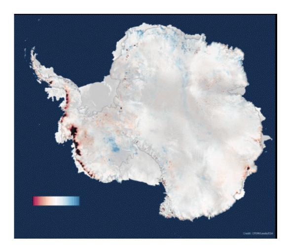
Three years of measurements from CryoSat-2 show that the Antarctic Ice Sheet is now losing 159 Gigatons of ice each year, enough to raise global sea levels by 0.45 millimetres per year. Colour scale ranges from -1 to +1 metres per year. Credit: University of Leeds
