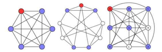
In a complete graph (left) every node is connected to every other. For other well studied graphs, the Paley graph in the center and the Latin square graph on the right, that is not true. A quantum particle could hop directly to the target position, in red, only from connected nodes, marked in blue. Credit: Tom Wong, UC San Diego
