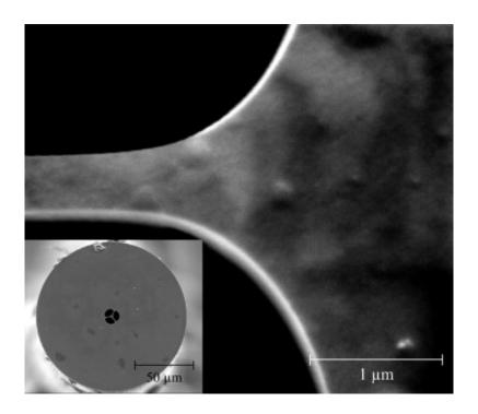
SEM image of the inner walls of a F2 suspended core fiber internally coated with MEH-PPV. The inset shows a wide-angle view of the same fiber. Credit: *Sensors and Actuators B: Chemical*, Volume 199, August 2014, Pages 22-26, ISSN 0925-4005, DOI: 10.1016/j.snb.2014.03.031.
