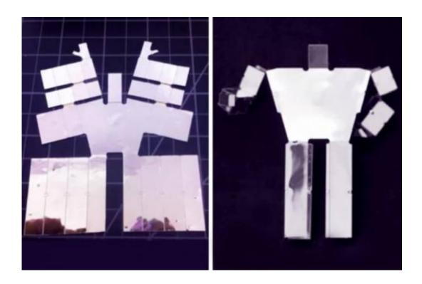
Before-and-after stills from the video, "An End-to-End Approach to Making Self-Folded 3D Surface Shapes by Uniform Heating." The left image shows the self-folding sheet for a humanoid shape while the right image shows the completed self-folded humanoid shape.
