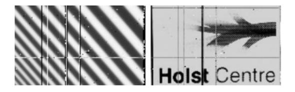
Examples of X-ray image (left) and optical image (right) obtained with Holst Centre's X-ray detector on plastic substrate.
