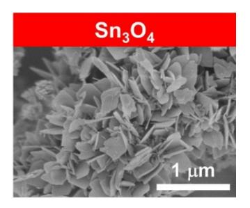
Figure 1 from the press release material. Electron microscope imagery of Sn3O4 catalyst. The synthesized material is a collection of microsized (one millionth of a meter) flaky crystals.
